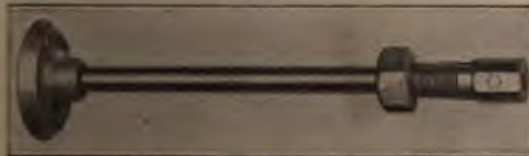
The Lack of a Center Hole in the Valve Stem is Overcome by the Use of a False Center
